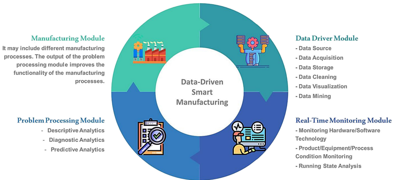
Fig. 1 The four modules of data-driven smart manufacturing according to [8]. The data collected from the manufacturing processes should be pre-processed and analyzed and be used for real-time monitoring of the manufacturing processes. The running state analysis may provide insight
