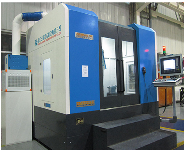
Fig. 5 Experimental platform of seven-axis six-linkage adaptive CNC abrasive belt grinder
