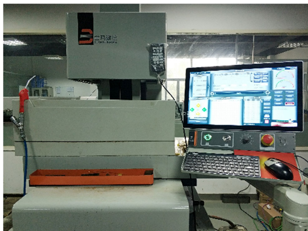
Fig. 2 The fast EDM drilling machine tool used in the experiments
