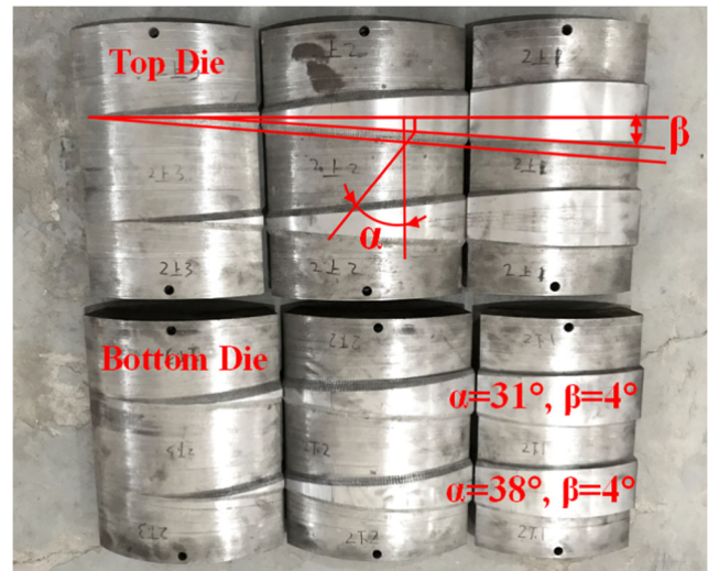
Fig. 4 Forming wedge tools of \alpha = 31^\circ and \alpha = 38^\circ with the same \beta = 4^\circ
