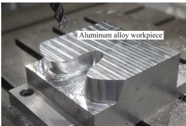
Fig. 20 Machining results of five-axis toolpath by the proposed feedrate-scheduling algorithm
