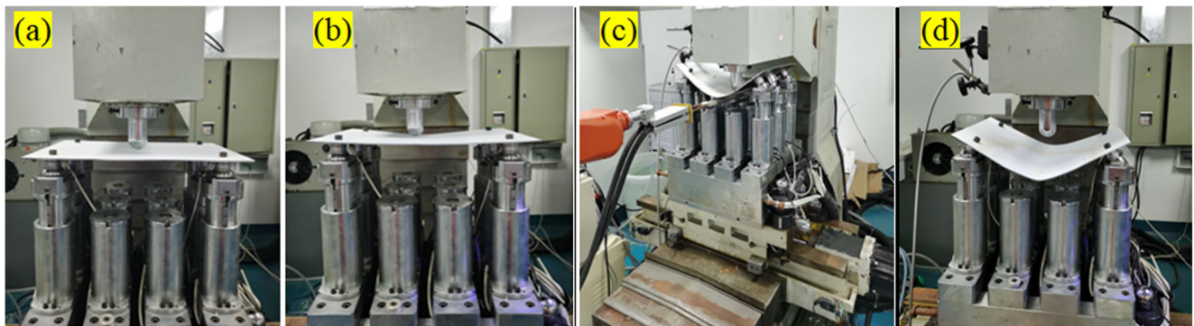
Fig. 15 Experimental plates at various states. a Initial state. b First punching state. c Middle heating state. d Last state
