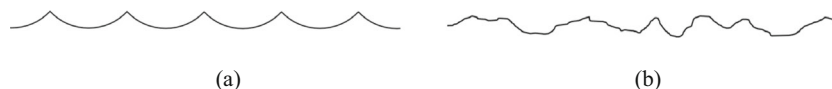
Fig. 11 a Simulated profile from an unworn tool. b Simulated profile from a worn tool
