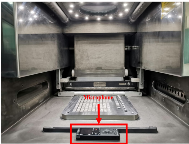
Fig. 16 The system of acoustic signal acquisition (Schematic diagram)
