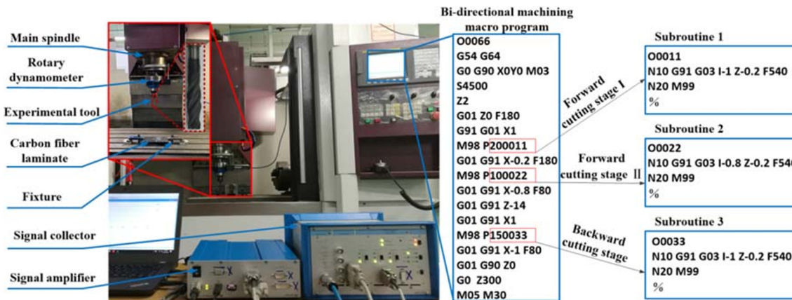
Fig. 2 The experimental site and macro program of hole making by bi-directional helical milling
