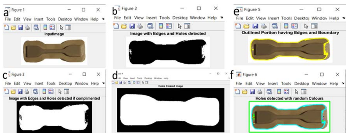
Fig. 6 Processing steps of pore's detection for an image without defect. (a) Input image. (b) Complemented image of a sample. (c) Binary image of sample exposing every defect. (d) Complemented images of samples
