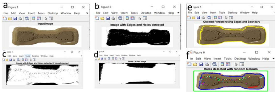
Fig. 5 Processing steps of pore's detection for an image with defect (a) Input image. (b) Complemented image of a sample. (c) Binary image of sample exposing every defect. (d) Complemented images of samples
