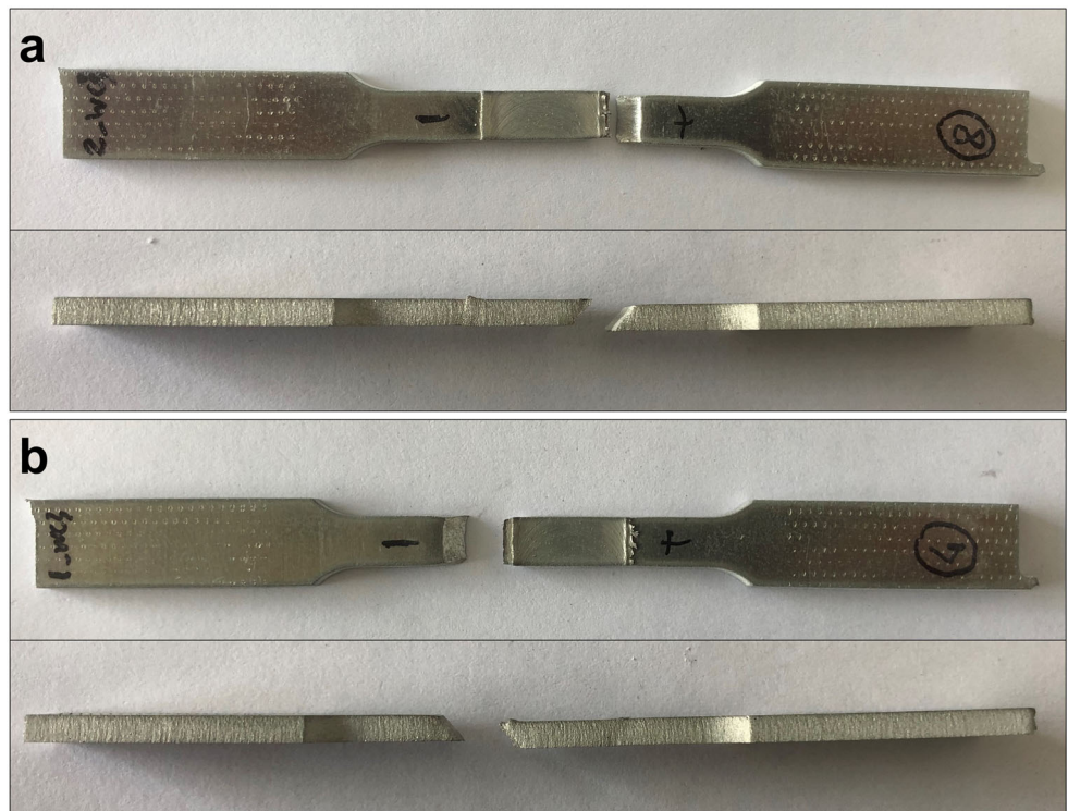
Fig. 10 Typical fracture locations of friction stir welding joints: a advancing side (+), b retreating side (-)
