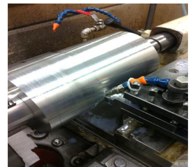
b) Arrangement of MQL Nozzles
