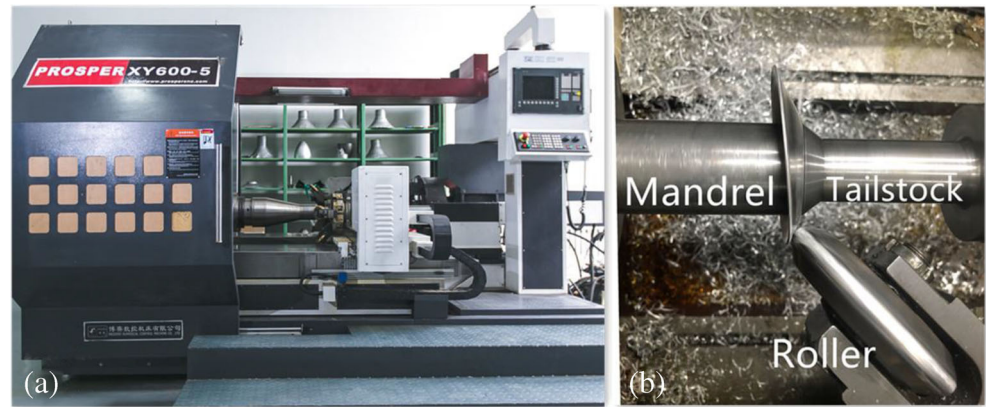
Fig. 1 PS-CNCXY600-5 NC spinning lathe: a full view of the lathe and b working portion of spinning
