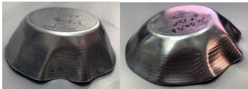
Fig. 26 Examples of failed products using the rotational pass set
