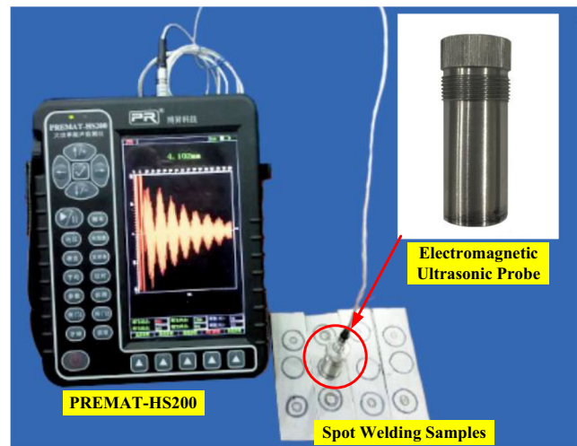
Fig. 11 The electromagnetic ultrasonic testing equipment
