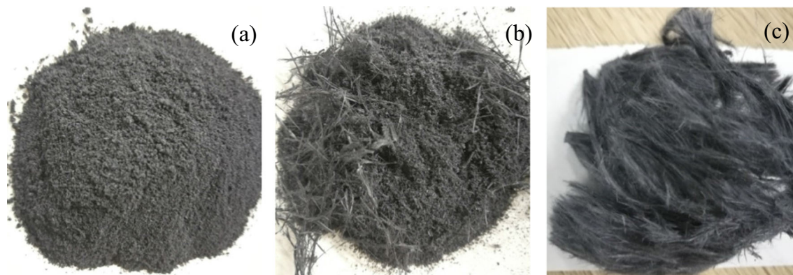
Fig. 13 The chip type of CFRP: (a) powdered chips, (b) mixed chips, and (c) floc-shaped chips
