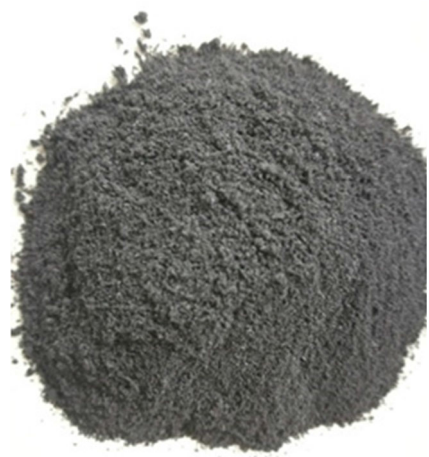
Fig. 4 Powdered chips during the turning of CFRP bars
