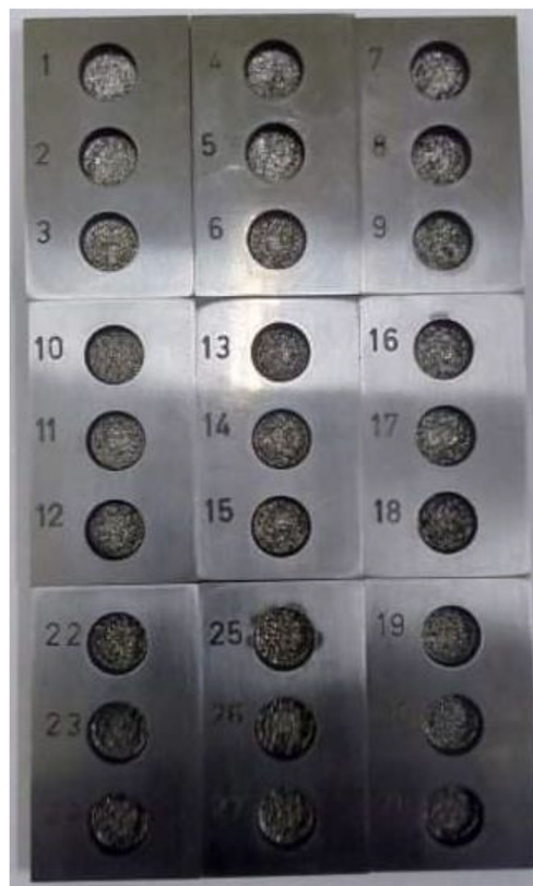
Fig. 9 Workpieces used in the tests after machining
