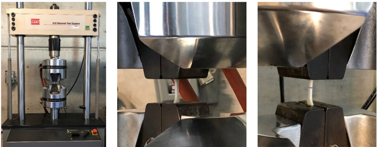
Fig. 2 From left to right: MTS 810 material testing system, specimen before the test, specimen after the test
