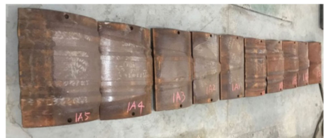
Fig. 8 The manufactured die of the H630 machine
