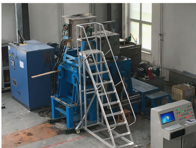
Fig. 2 The \phi 500 \times 350 mm twin-roll strip micro-vibration cast-rolling mill used herein
