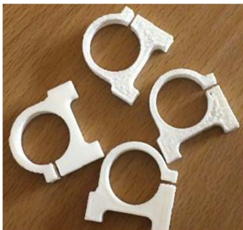
Fig. 10 The 3D printed models (fire extinguisher mounts)
