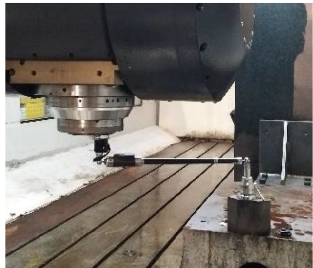
Fig. 18 Initial installation of DBB measurement system
