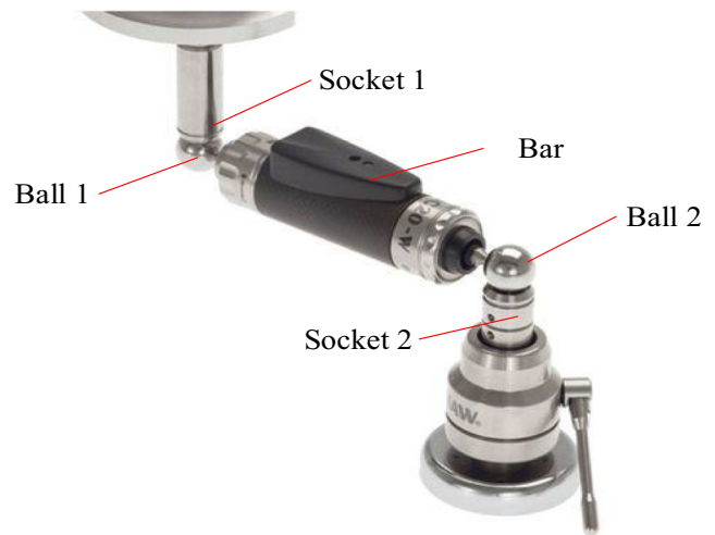
Fig. 13 Structure of double ball-bar
