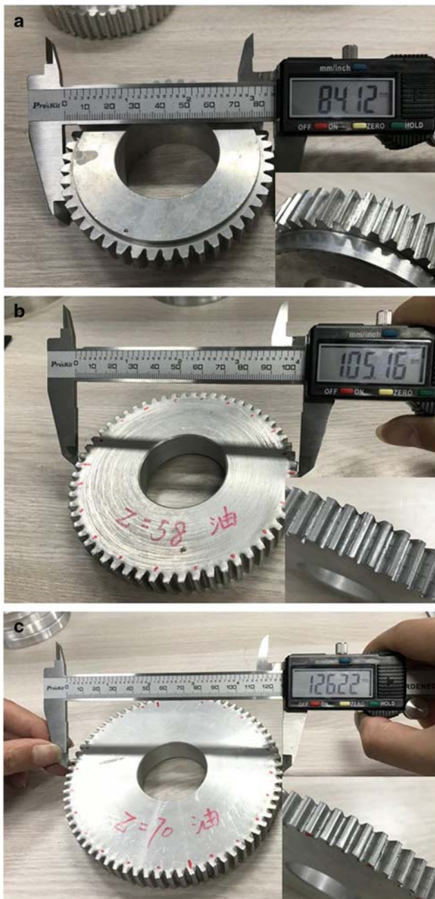
Fig. 17 Top circle of the formed gears with different number of teeth: a z_2 = 46 ; b z_2 = 58 ; c z_2 = 70
