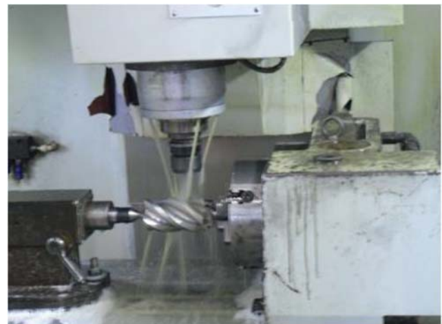
Fig. 13 Screw rotor machining process
