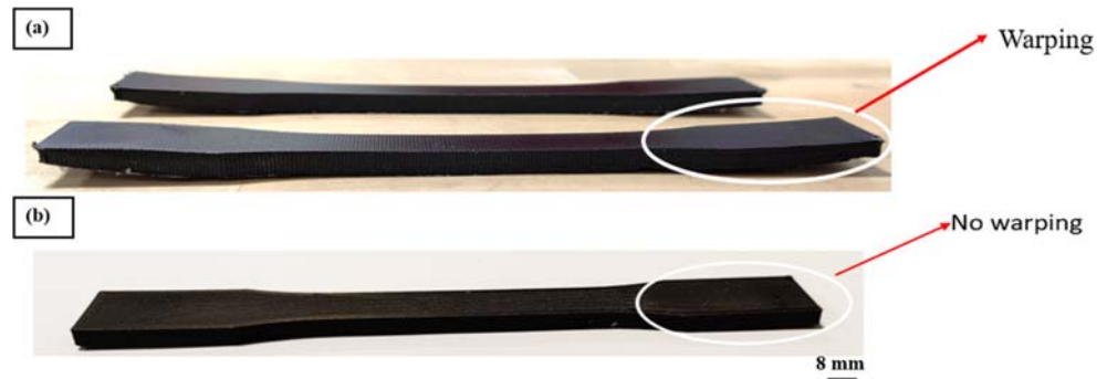
Fig. 2 PC/SCF specimens printed using a no closed chamber b closed chamber
