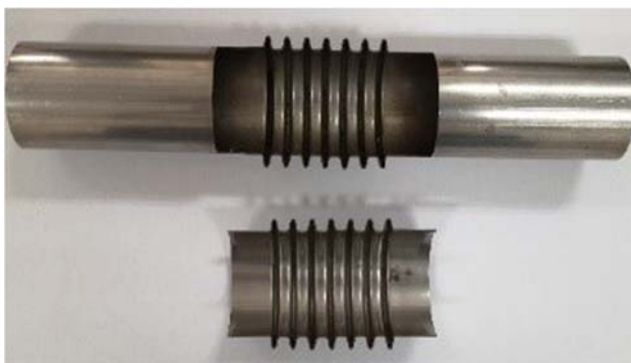
Fig. 21 Hydroforming bellows and two halves
