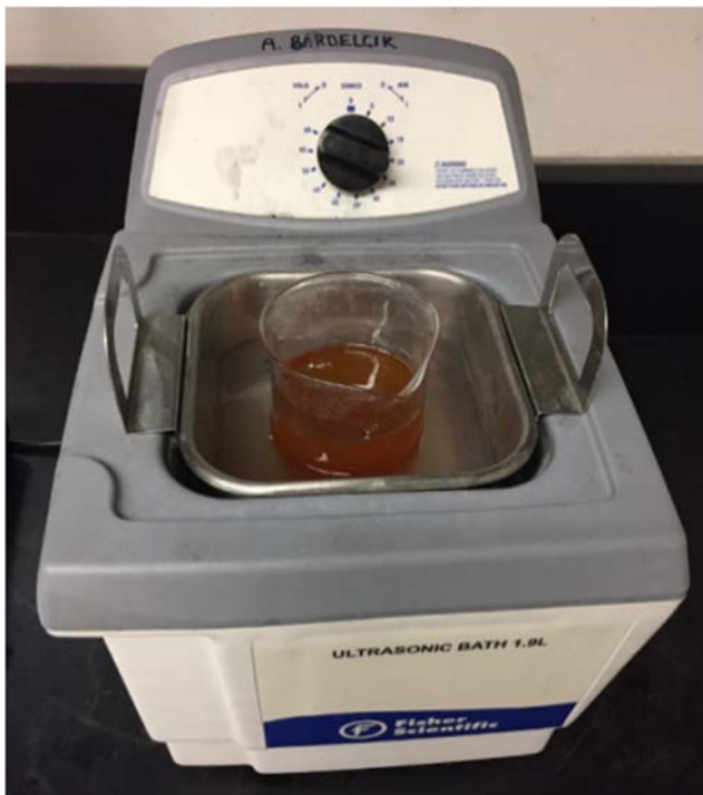
Fig. 2 Image of ultrasonic bath 1.9-L device used to achieve dispersion
