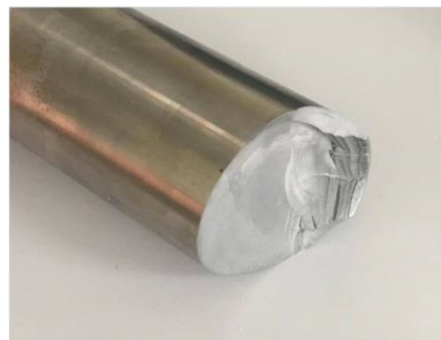
Fig. 20 Punch fracture surface
