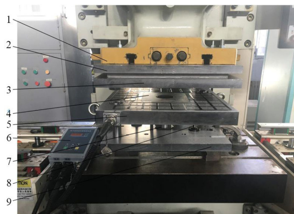
1 Press slide, 2 Upper base, 3 Suction plate and die, 4 Blank holder, 5 EPM chuck, 6 Controller, 7 Punch, 8 Nitrogen spring, 9 Lower base
