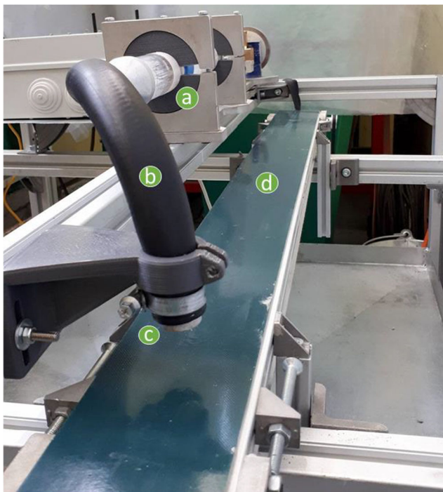
Fig. 5 Image of the experimental apparatus. a Extruder system. b Pipe. c Nozzle. d Conveyor belt
