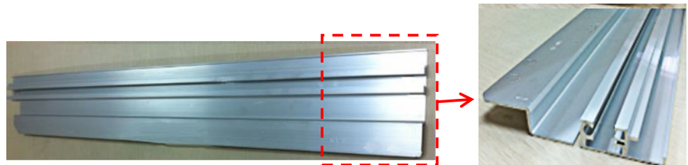
Fig. 21 Sample of the large-size, flat-wide, and thin-walled aluminum profile using optimal die
