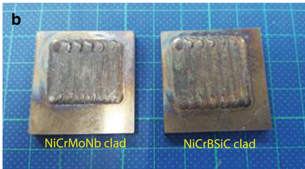
Fig. 2 a Schematic of laser cladding process and b samples after laser cladding
