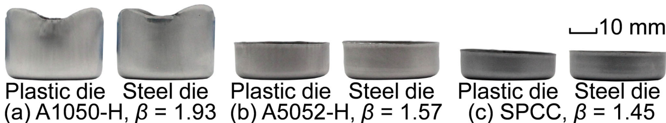
Fig. 15 Drawn cups with plastic and steel dies for press oil
