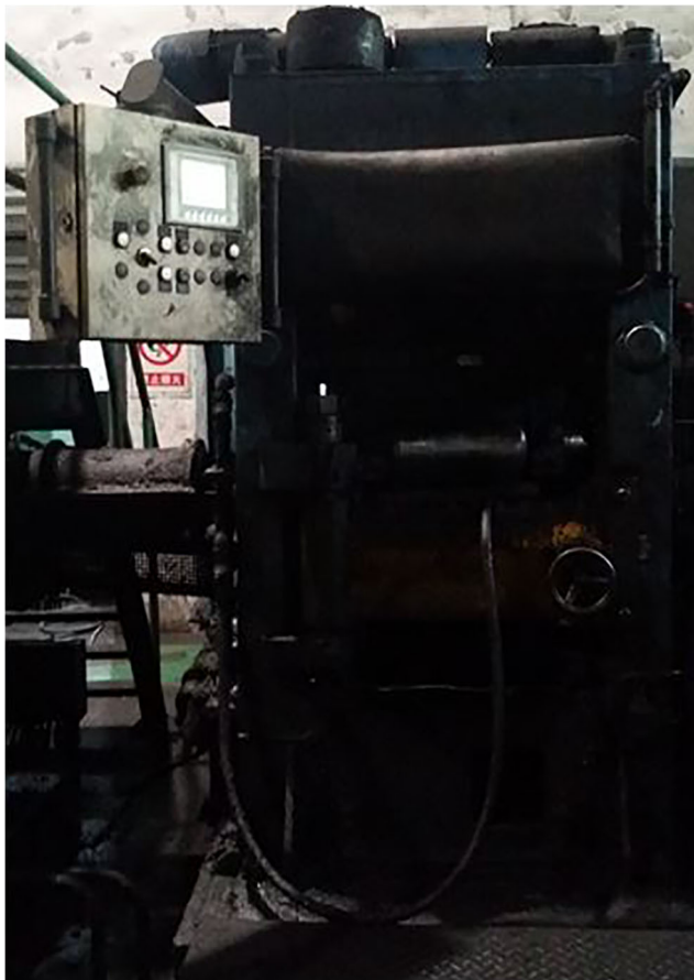
Fig. 21 Straightener for a factory
