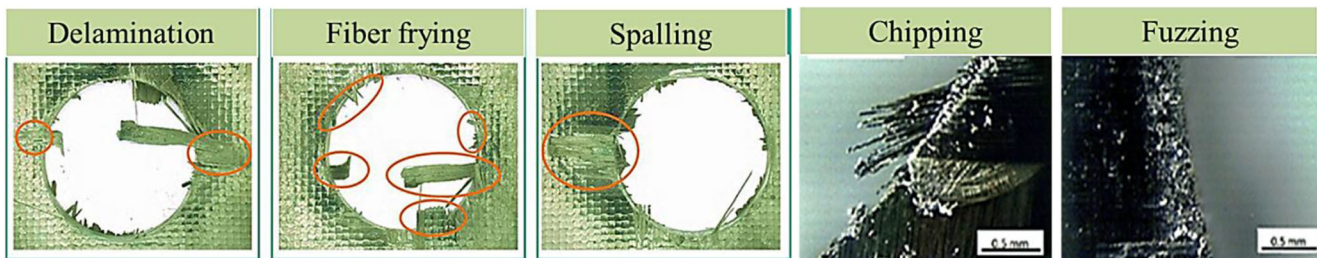
Fig. 2 Drilling induced hole damage in FRPs [17]
