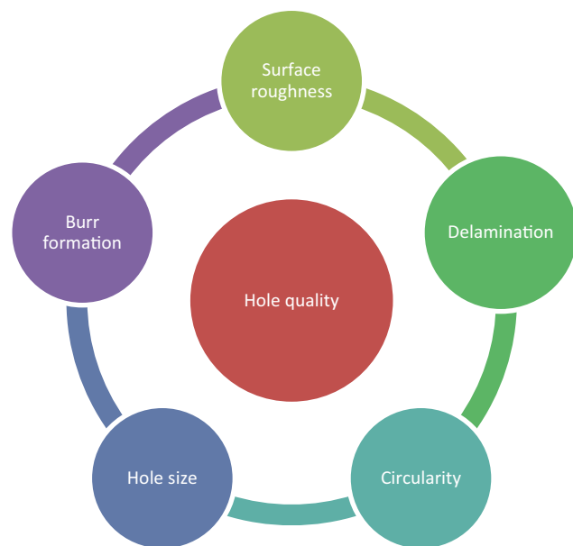
Fig. 5 Hole quality inspection criteria [51]
