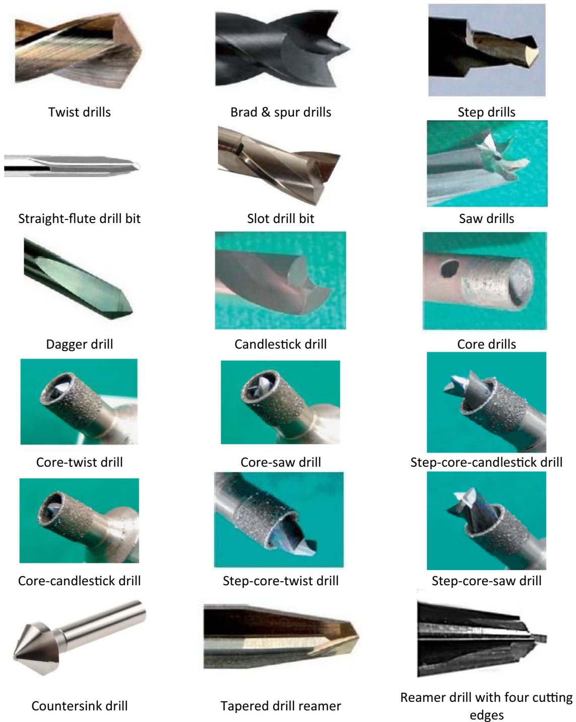
Fig. 10 Drill tool geometries used in CFRP [30,31,33,36,37,38,62,91,98,101,102,103,104,105,106,145,146,147]
