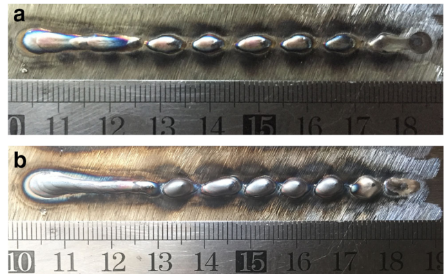
Fig. 8 Forming appearances of discontinuous beads, a Exp. No. 6, b Exp. No. 19
