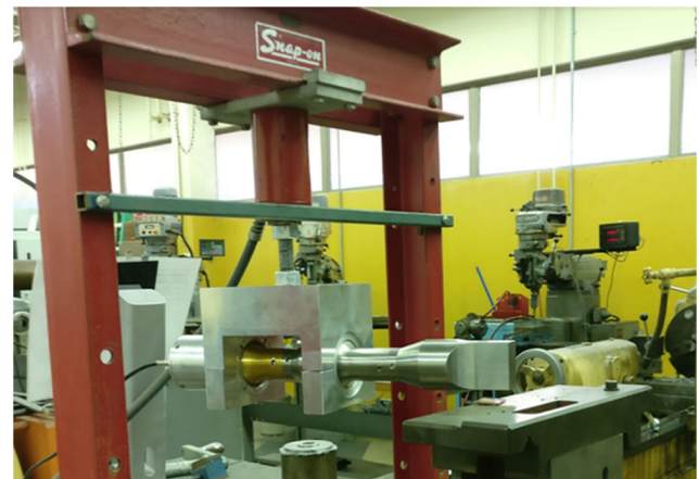
Fig. 3 In-house built experimental setup of UAM on CFRP/Ti stacks [14]
