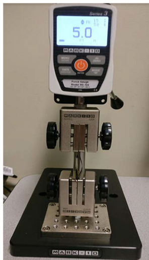
Fig. 20 Lap shear testing of CFRP/Ti substrates
