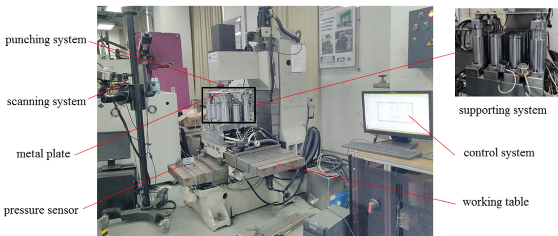
Fig. 2 Experimental setup of incremental bending process
