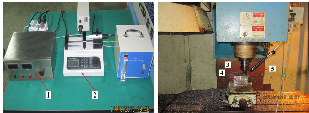
Fig. 1 Photographic view of electrostatic atomization milling system: 1, high-voltage electrostatic generator; 2, syringe pump; 3, cutting tool; 4, workpiece; 5, nozzle
