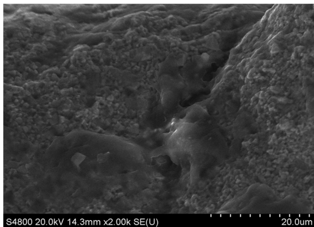
Fig. 8 SEM micrograph of thermal crack under NFEAL condition
