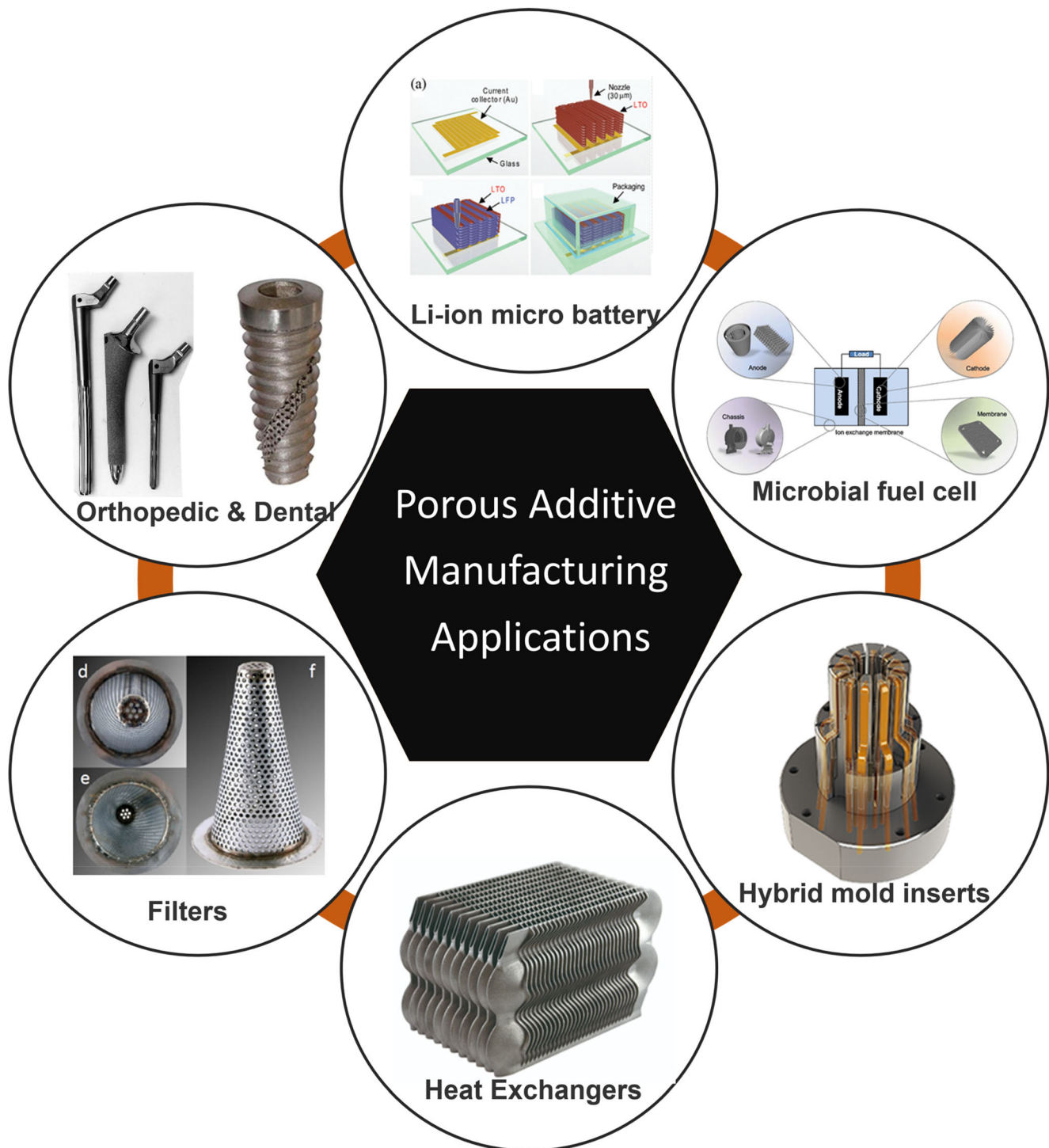
Fig. 13 Next generation of application of porous materials using AM technologies: a 3D printing of interdigitated Li-ion microbattery architectures [69]; b 3D-printed components of microbial fuel cells
