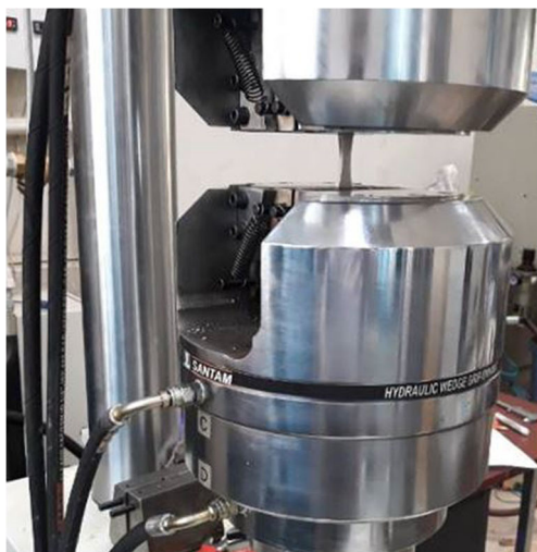
Fig. 5 High-cycle fatigue test on a specimen
