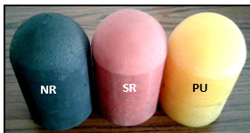
Fig. 7 Elastomeric punches used in the flexible bulging with radius of 35 mm
