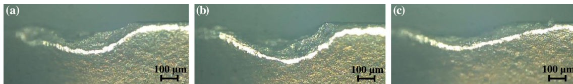
Fig. 17 Microscopic images of the flank wear using a oil-based MQL, b \text{Al}_2\text{O}_3 fluid MQL, and c \text{Al}_2\text{O}_3 fluid EMQL with -4 kV (flow rate 20 mL/h, air pressure 0.3 MPa, cutting speed 100 m/min, feed rate
