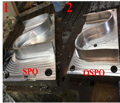
Fig. 18 Two test pieces produced using the SPO
