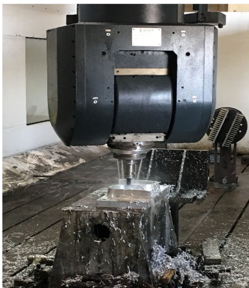
Fig. 17 S-shaped test piece being machined
