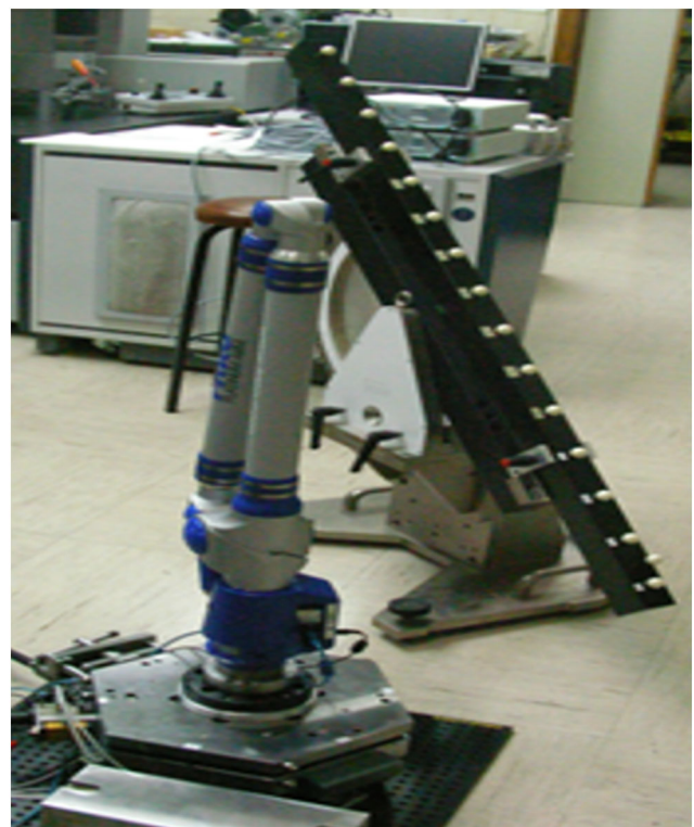
Fig. 7 Test position Diag45Downward_Orientation used in the evaluation process
