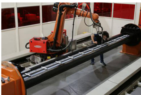
Fig. 19 Cranfield University's WAAM 3D printer being used to print a double-sided, 6-m long aluminum spar [139]
