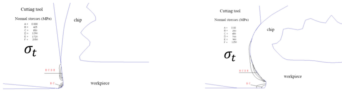
(a) Normal Stress distribution of the tool (KT=0)
