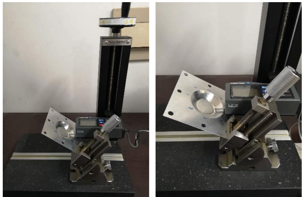
Fig. 24 Roughness measurement. a Point-pressing incremental forming. b Consecutive incremental forming
