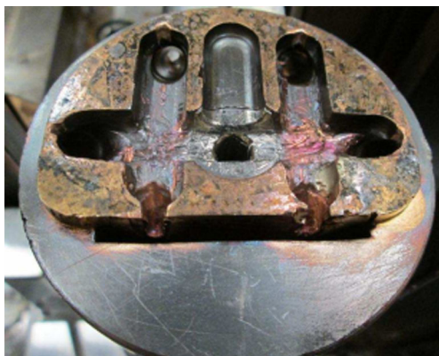
Fig. 4 Wear of the Ampcoloy 83 mold insert at the injection gate
