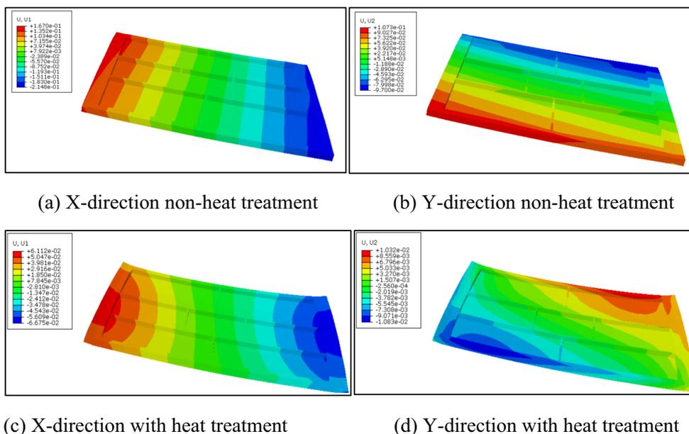
**Fig. 5** Residual stress— $\sigma_{xx}$  comparison in finishing process
