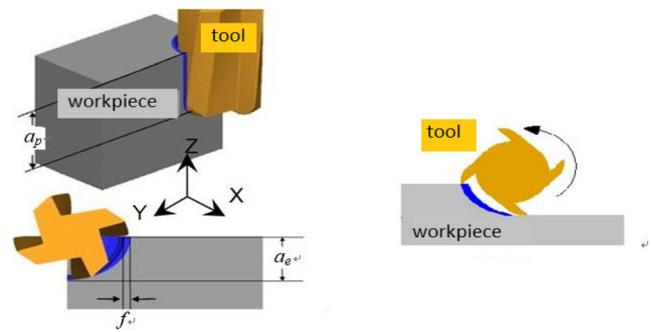
Fig. 1 Simulation model of milling process (Third Wave Systems, 2010).
