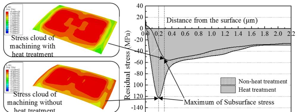
**Fig. 3** Residual stress— $\sigma_{yy}$  comparison in semi-finishing process
