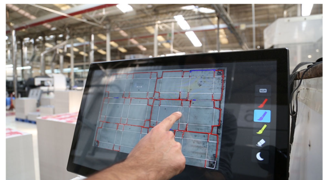
Fig. 13 Manual edition of a digitization of a correction template
